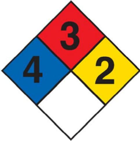
The NFPA 704 hazard rating label for epichlorohydrin, at left, includes a "4" for the blue health hazard, the highest rating, meaning the hazard can be lethal. The red flammability hazard is a "3," meaning it can be ignited under almost all ambient temperatures. The yellow instability hazard is rated as a "2," meaning violent chemical change is possible at high temperatures or pressures. The white special hazard space is empty because the compound poses no special hazard.
